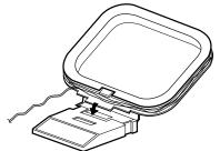
Attach the AM loop to its base by snapping the tabs on the loop into the slot in the base.
